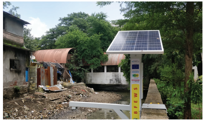
IoT based early warning sensors for urban flooding & water logging installed at Thana College, Thane
